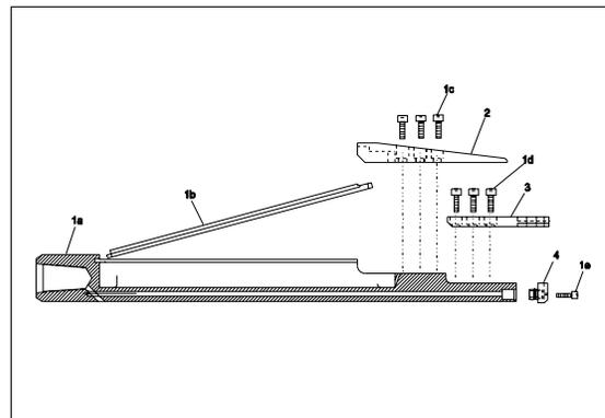
Apply thread lube to the male end of the drill pipe. Attach the drill head assembly by screwing it on the drill pipe and tighten with hand wrenches.
