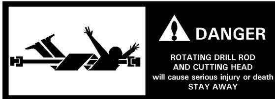
**▲ WARNING** Moving parts can cut off hands, feet, or fingers. **DO NOT TOUCH MOVING PARTS.**
