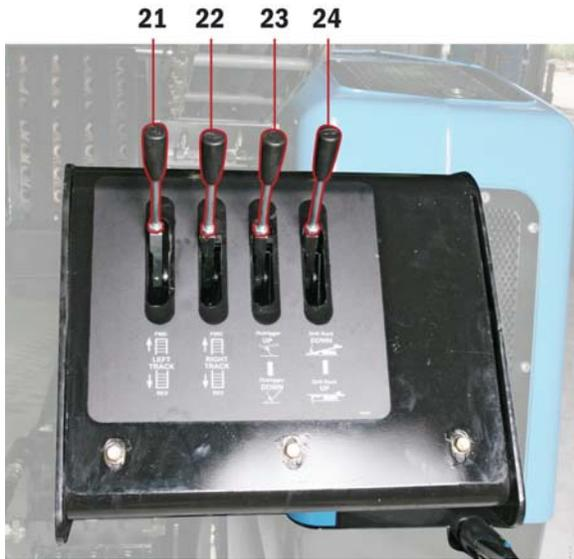
**21. Left Track:** Track Control: Move the handle forward to drive forward and back to drive in reverse. Combinations with left and right track control path and direction.
