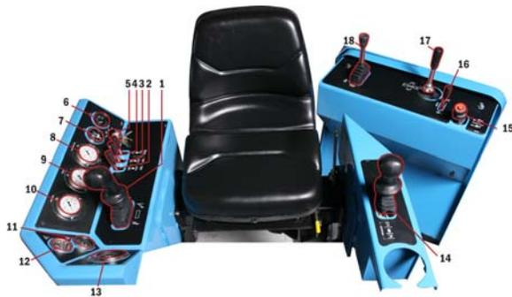
**1. Thrust Control:** Controls drilling (push for forward thrust) and back reaming (pull for rear thrust)
