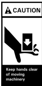
**IMPORTANT** Clear all persons and tools from around the drill pipe before starting operation and during operation, keep bystanders at least 10 ft (3 m) away from drill. Do not stand over trench or drill pipe while drilling.
