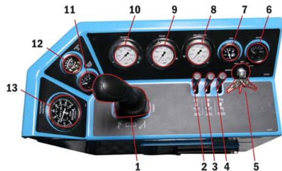
**5. Ignition Switch:** This handle has four positions to control the operation of the engine.
