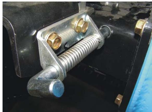
In order to provide maximum protection for the hydraulic safety override seat switch while tramping or transporting the drill, a locking mechanism is provided to secure the seat in the up position.
