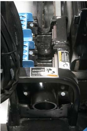
Then slowly thrust forward until the front (male) end of the pipe is in the jaws of the makeup wrench. Tighten the section of drill pipe onto the saver sub by locking the makeup wrench. Using forward rotation, rotate pipe until it is tightened to full drill rotation torque.
