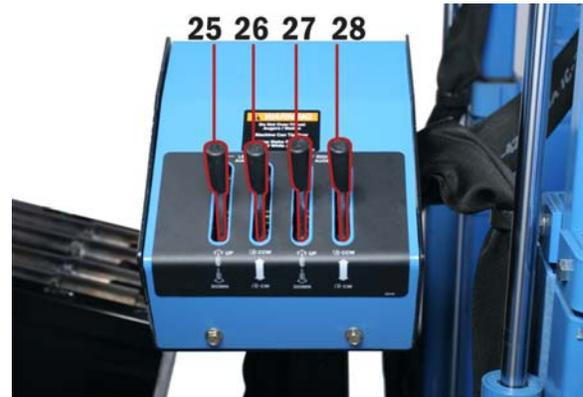
**25. Left Auger Raise/Lower:** Pull handle to lower auger. Push handle to raise auger.
