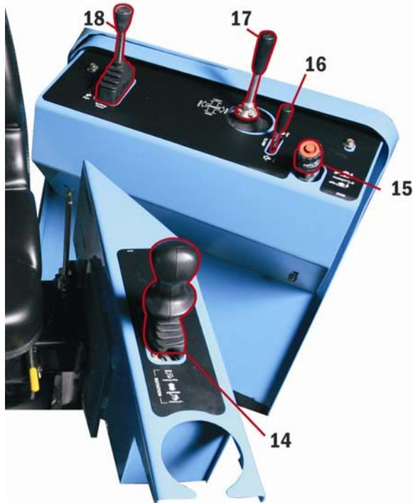
**14. Rotation Control:** Pull joystick for clockwise (drilling) rotation. Push joystick for counter-clockwise (breakout) rotation.
