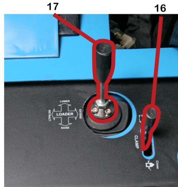
**17. Loader:** Move toward pipe rack to extend pipe loader, move away from drill to retract. Pull toward operator and move loader down; push away from operator to raise.
